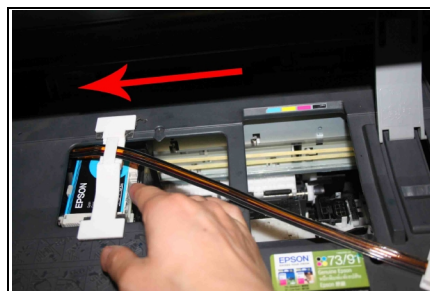
Move the carriage to the leftmost and rightmost to make sure that the tube can be straight.
