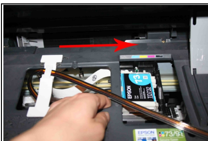
Move the carriage to the leftmost and rightmost to make sure that the tube can be straight.
